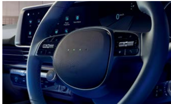
Interactive LED Steering Wheel* Four Interactive Pixel Lights on the steering wheel and LED lights on the crash pad indicate various car statuses (welcome/goodbye, voice recognition, etc).
