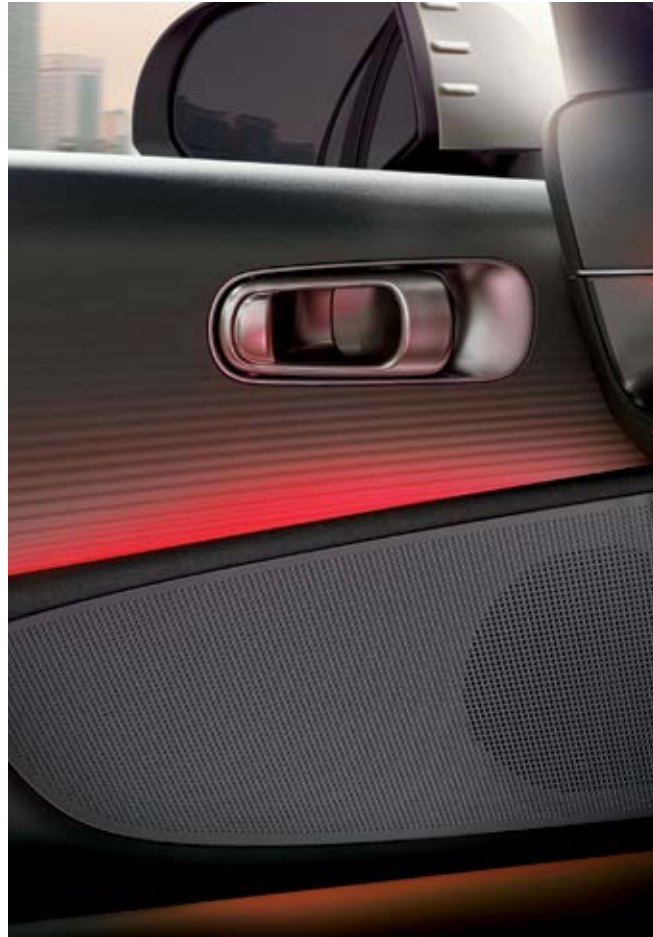
Speed Sync Lighting* To enhance the dynamic driving experience, the ambient light's brightness adjusts from 10% at 30 km/h to 100% at 100 km/h.
