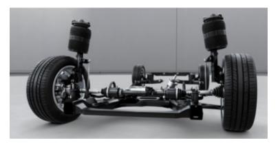
No matter if you are on the motorway or a track with ruts: the **AIRMATIC** air suspension can adjust the suspension to suit the road surface. Damping can be regulated for each individual wheel automatically – to suit the current driving situation and the state of the road.
