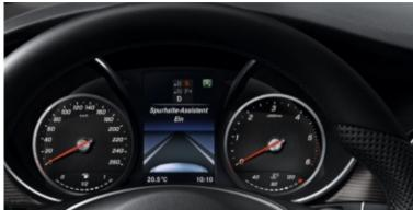
The **standard Driving Assistance Package** promotes safe and relaxed driving by means of the 3 intelligent systems Active Brake Assist, Lane Keeping Assist and Blind Spot Assist. As a result, it can help to avoid accidents or reduce their consequences.
