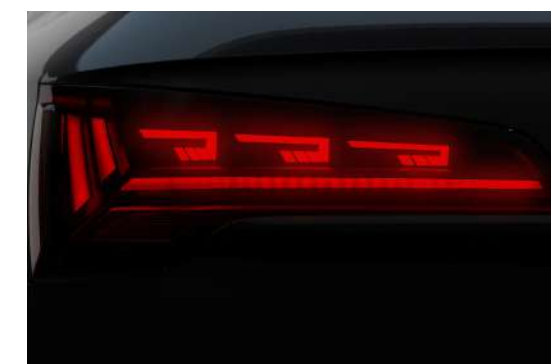
OLED rear lights with specific rear light signature 1
