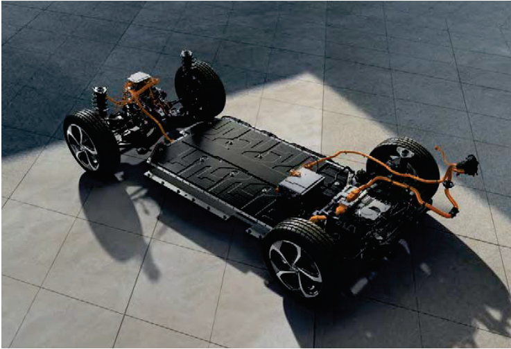
Electric Global Modular Platform (E-GMP). The Kia EV6 is the first vehicle based on the Kia E-GMP platform. The new long-wheelbase platform is a clean slate. It introduces a flat floor, facilitating new comfort and utility choices. Its modularization permits more flexible development to secure performance, maintenance and safety objectives. Performance benefits include greater power, driving range and control, as well as shorter charging times.
