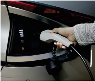
Charging port. The charging port door opens and shuts electronically. Just press the door itself, or the button on the left of the dash controls. Inside the cover, a bar graph displays the charging level.
