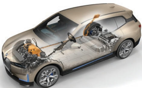
BMW 5 th generation eDrive with two motors
