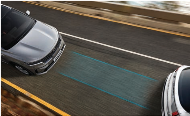
Smart Cruise Control (SCC) (SX Tech Pack & GT Tech Pack only) With a simple touch of a button, SCC will maintain the driver's selected speed. Using the front view camera and front radar, the system allows the vehicle to automatically maintain a safe following distance, reduce speed, and even come to a complete stop and start again, if necessary.
