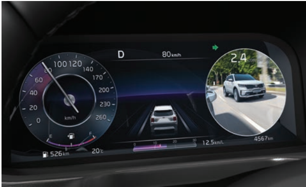
Blind-spot View Monitor (BVM) (SX Tech Pack & GT Tech Pack only) Activate the turn signal and BVM will present live video footage on the instrument cluster of other vehicles in the blind spot on the side of the intended lane change.
