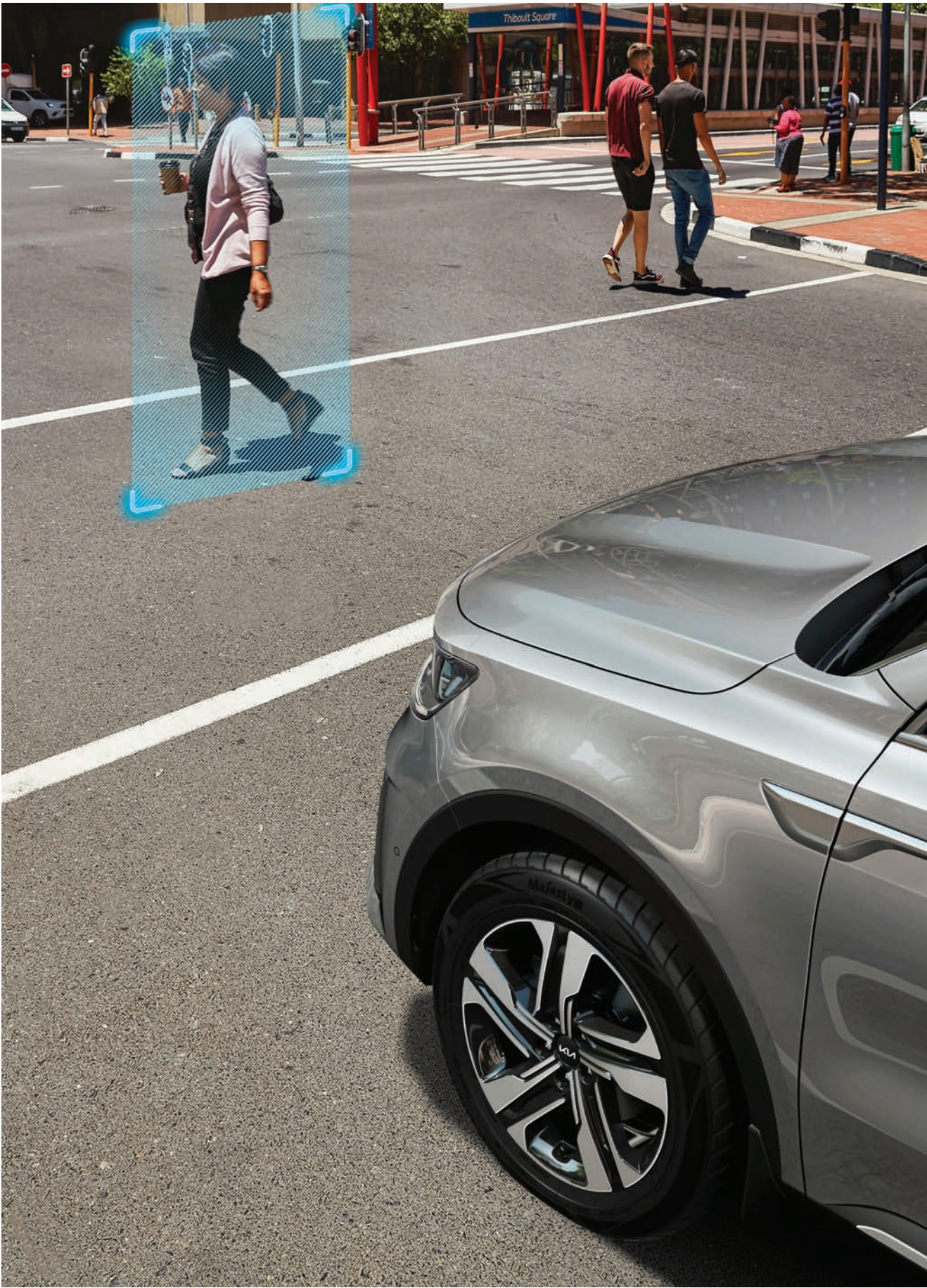
Forward Collision-avoidance Assist (FCA) (SX Tech Pack & GT Tech Pack only) FCA uses a front view camera and front radar to detect vehicles, pedestrians or cyclists ahead. By warning and braking automatically, it can help you avoid or reduce the severity of an accident.
