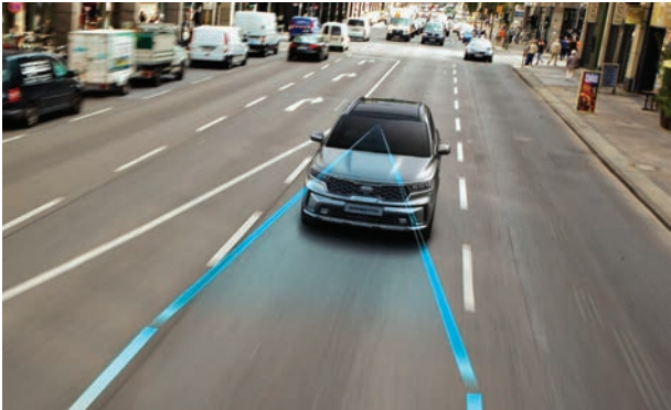
Lane Keeping Assist (LKA) (SX Tech Pack & GT Tech Pack only) There's no need to worry about drifting out of your lane. LKA monitors your position in the lane, and if you begin to wander to either side, it alerts you and even steers you back into place to keep you precisely where you need to be.
