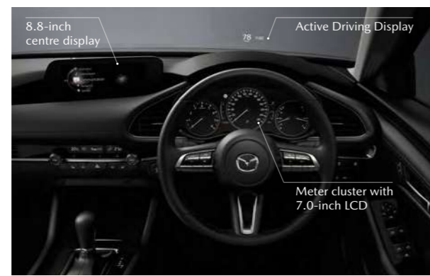
Active Driving Display This windscreen-projected display is close to your line of sight for easy visibility. Important driving information is displayed in the upper section, vehicle status information is displayed in the lower section.
