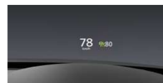
Active Driving Display This windscreen-projected display is close to your line of sight for easy visibility. Important driving information is displayed in the upper section, vehicle status information is displayed in the lower section.
