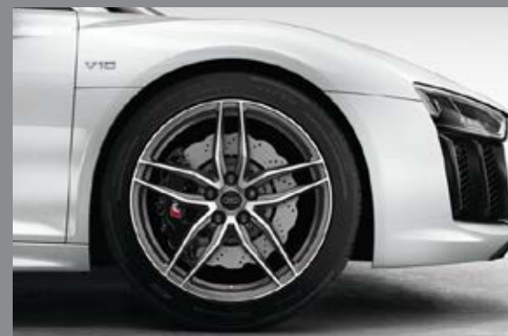
Forged aluminium alloy wheels, 5 twin-spoke design, matt titanium look machine polished with R8 brake system
