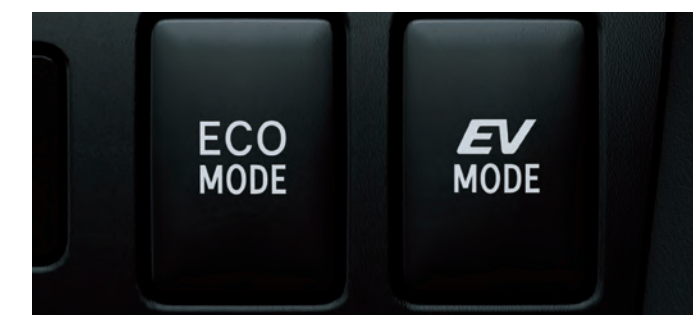
DRIVE MODE SELECTION FLEXIBLE FUEL ECONOMY Two levels of efficiency can be chosen, ECO mode or the environmentally friendly EV mode, which uses the electric motor only.
