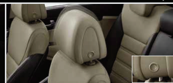
One-button adjustable headrest The 1st-row seats have headrests that offer up, down and sliding adjustments with the simple push of a button.
