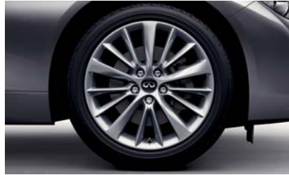
18 X 7.5-INCH ALUMINIUM-ALLOY WHEELS WITH ALL-SEASON RUN-FLAT TYRES
