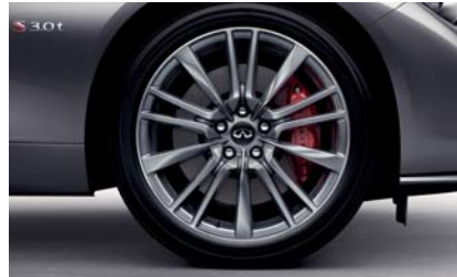
19 X 8.5-INCH ALLUMINIUM ALLOY WHEELS WITH RUN-FLAT PERFORMANCE TYRES
