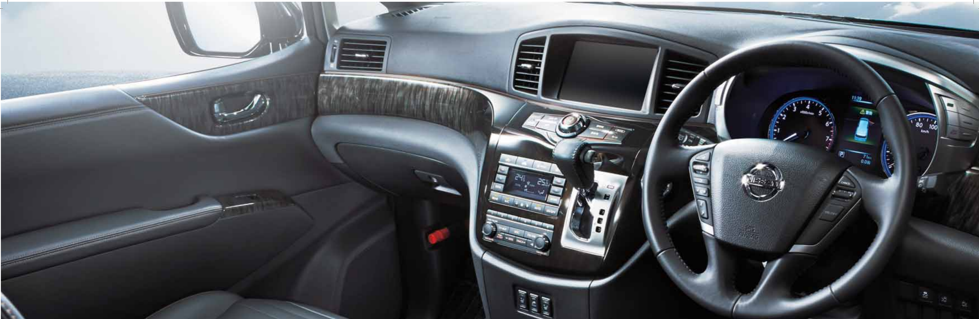
AUTOMATIC DUAL ZONE AIR CONDITIONING SYSTEM features Plasmacluster nano e-ion technology which emits positive & negative ions, effectively cleaning and refreshing the cabin air. Independent controls for the right and left zones allow both the driver and passenger to personally adjust the temperature. The rear passengers also have an independent control allowing them to adjust the temperature for utmost comfort.
