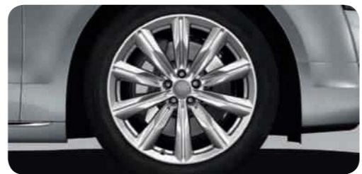
Cast aluminium wheels in 10-spoke star design size 9 J x 20 with 265/40 R 20 tyres 1
