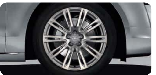
Forged aluminium winter wheels in 10-parallel-spoke design size 9 J x 20 with 265/40 R 20 tyres 1 , permissible top speed 240 km/h, cannot be fitted with snow chains
