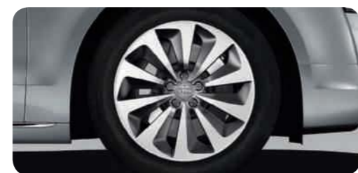
Cast aluminium wheels in 10-arm turbine design (hybrid design), contrasting grey, partly polished 2 size 9 J x 19 with 255/45 R 19 tyres 1 . Available only for the A8 hybrid and A8 L hybrid
