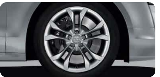
Cast aluminium winter wheels in 5-parallel-spoke design (S design) size 9 J x 20 with 265/40 R 20 tyres 1 , permissible top speed 240 km/h, cannot be fitted with snow chains. Available only for the S8
