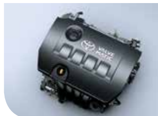
1.6L Dual VVT-i valvematic engine
